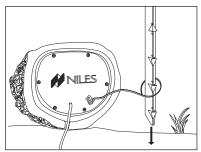
Figure 12 Security Stake Attachment to Cable
